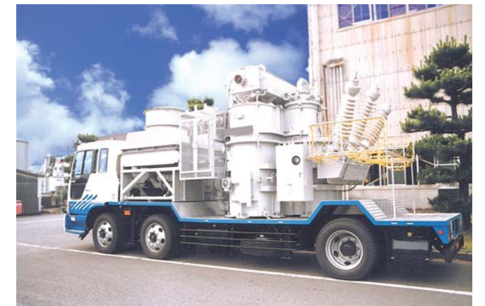
Mobile transformer 20MVA, 77/6.6kV
