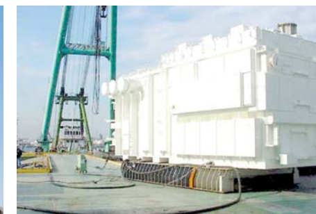
Arrival at the dock by using air castor.
