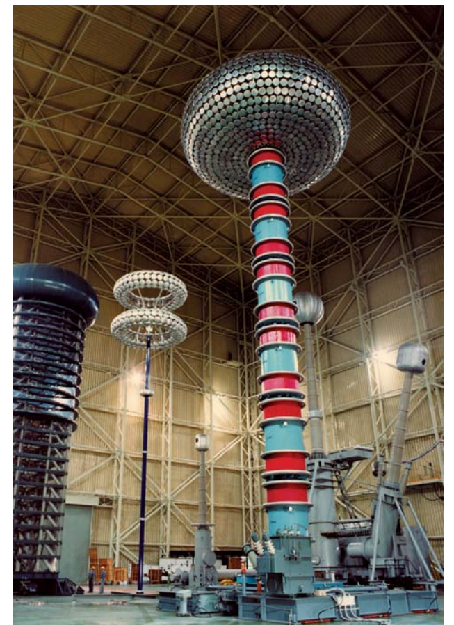
The laboratory has a 2,200kV AC generator and a 6,000kV impulse generator.
