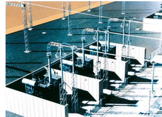
Single-phase shunt reactor 400MVAR, 800kV
