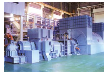
Short-circuit generator Voltage: 11.5/13.8kV Frequency: 50/60Hz Capacity: 250/350MVA Short circuit capacity: 3.0/3.6GVA
